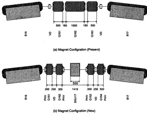
Figure 3: Creation of the short straight section.
