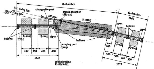
Figure 6: Conceptual chamber design in the bend section.
