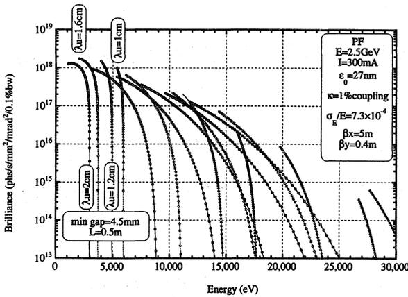
Figure 7: Example spectra of the radiation from short-period narrow-gap undulators.
