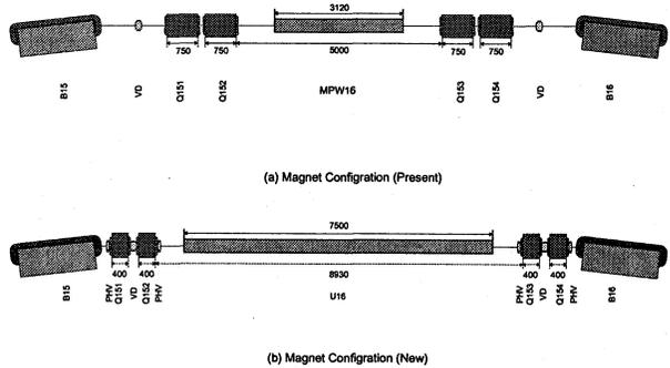
Figure 4: Extension of the long straight section.
