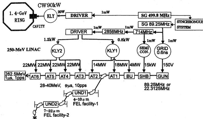
Fig.1 The schematic layout of the Saga-LS and rf systems for 1.4-GeV storage ring and 250-MeV linac.
