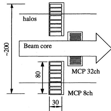
Figure 3: Schematic of MCP detectors. Center detector of 32 channel observes the core density profile. Others of each 8 channel are prepared to investigate the beam halos.
