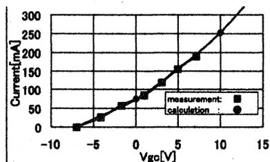
Figure 8: Measured and calculated peak currents as a function of the grid voltage.
