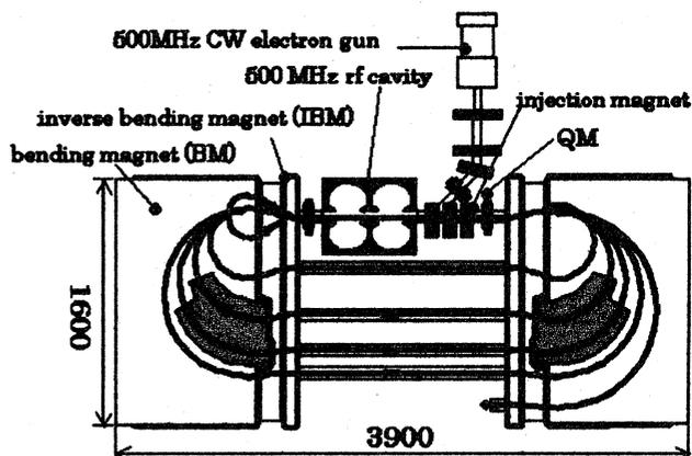
Figure 1: Schematic drawing of the 5 MeV cw microtron
