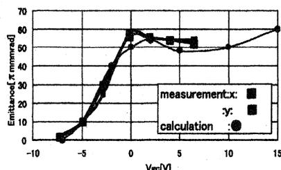
Figure 9: Beam emittances as a function of the grid voltage.
