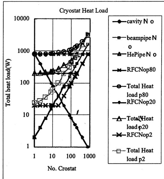
Figure. Static Cryostat Heat Load and No. of Cryostat.
