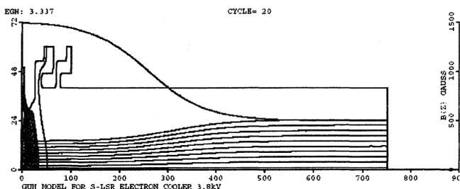
Fig.2 Simulation of electron beam trajectories during adiabatic expansion for  $B_{gun}=1.5kG$ ,  $B_{cool}=0.5kG$  and  $E_e=3.8keV$  (plot scales are not equal).
