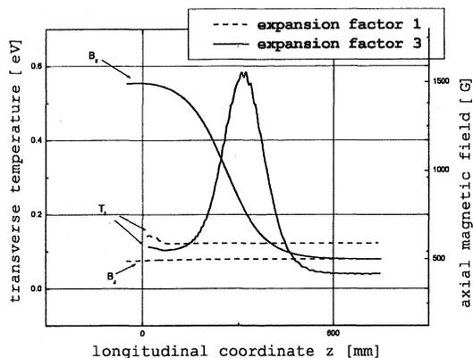
Fig.3 Effect of the adiabatic expansion on the transverse temperature of the electron beam.
