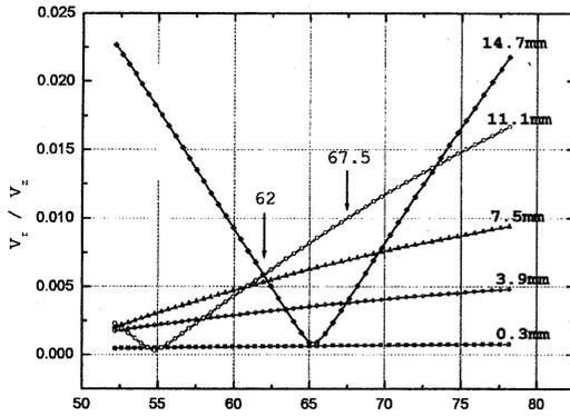
Fig. 4 Dependence of the radial electron velocity on the angle of the Pierce electrode ( $E_e=3.8\text{keV}$ ,  $B_{\text{gun}}=500\text{G}$ ,  $I_e=300\text{A}$ )
