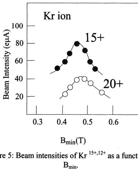
Figure 5: Beam intensities of Kr<sup>15+,12+</sup> as a function of B<sub>min</sub>.
