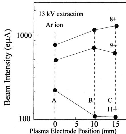
Figure 2: Beam intensity of Ar ions as a function of plasma electrode position.
