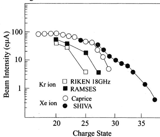
Figure 4: Beam intensities of Xe ions from SHIVA (closed circles) and CAPRICE (open circles) and Kr ions from RAMSES (closed squares) and RIKEN 18GHz ECRIS.
