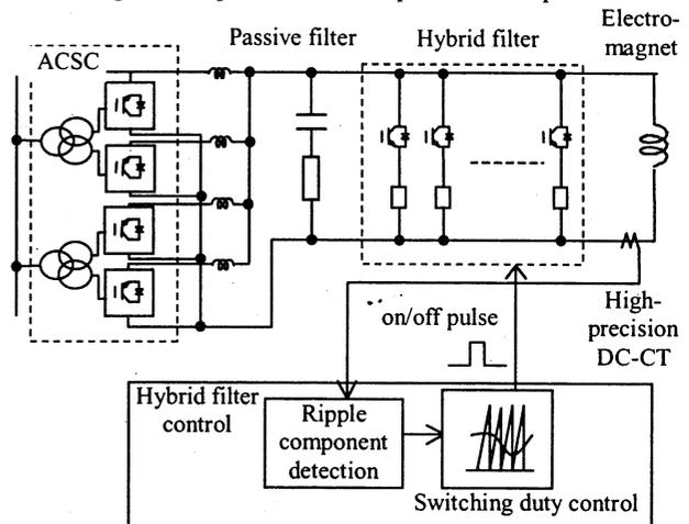
Figure 3 Prototype hybrid filter for mini-model
