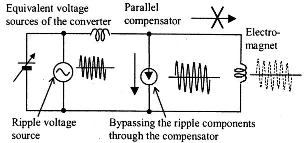
Figure 2 Operation of the parallel compensator
