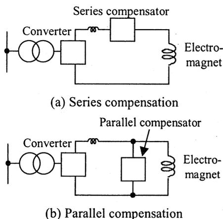
Figure 1: Ripple compensation methods
