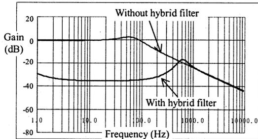
Figure 4 Frequency characteristics of hybrid filter
