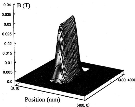
Figure 6: Magnetic field distribution of BM2
