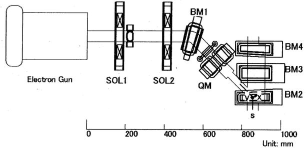
Figure 1: Schematic drawing of the LEBT of the CW microtron.
