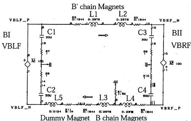
Figure 1: A schematic circuit of the bending magnet power supply system of the KEK PS 12 GeV main ring.
