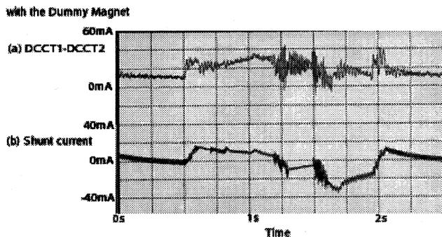
Figure 4: The difference between the B chain current and the B' chain current (upper line) and the ground shunt current (lower line) with the dummy magnet in the circuit.
