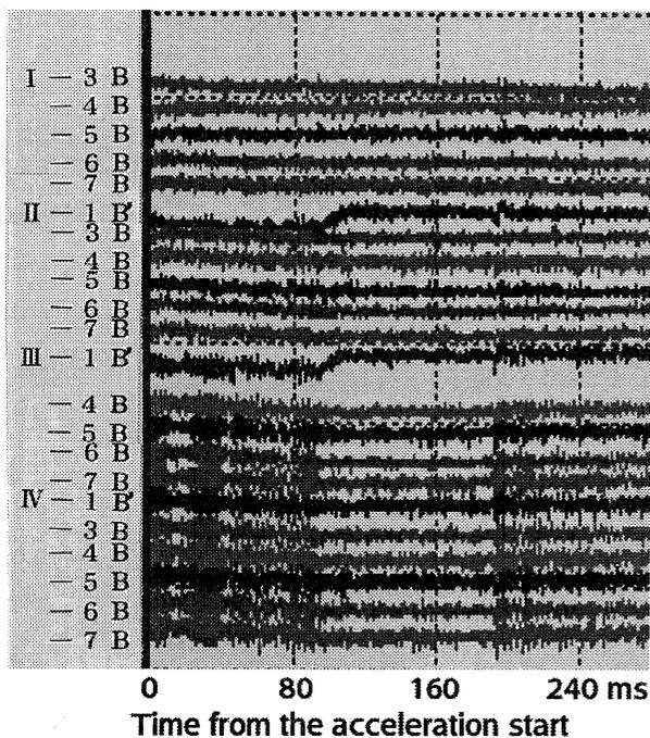
Figure 2: Backleg coil signals of the B chain magnets during the acceleration period.
