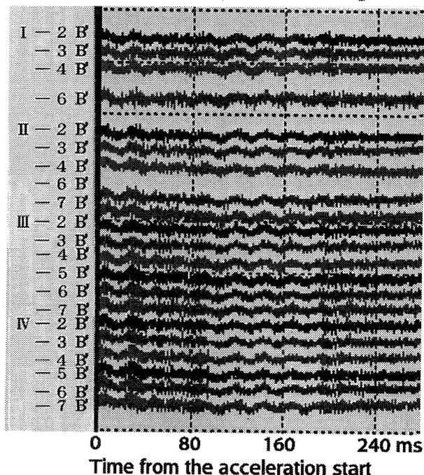
Figure 3: Backleg coil signals of the B' chain magnets during the acceleration period.
