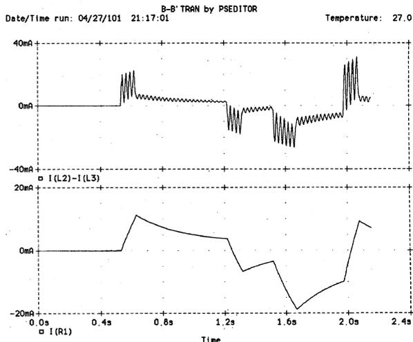
Figure 6: Circuit simulation results for the difference between the B chain current and the B' chain current (upper figure) and the ground shunt current (lower figure).
