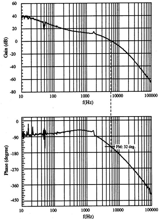
Figure 4: Bode diagram of the open-loop transfer function of the amplitude modulation, measured for the A3 cavity at the gap voltage of 180 kV. The horizontal axis represents the modulation frequency in Hz. The phase margin is 32 degree.
