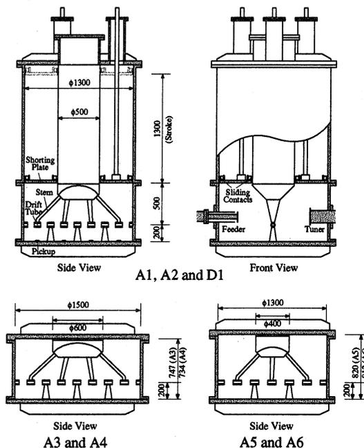
Figure 3: Schematic drawing of the CSM cavities.
