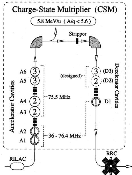
Figure 1: Conceptual drawing of the CSM. The cavities are represented by circles. The numbers in the circles indicate the “unit” of the CSM.
