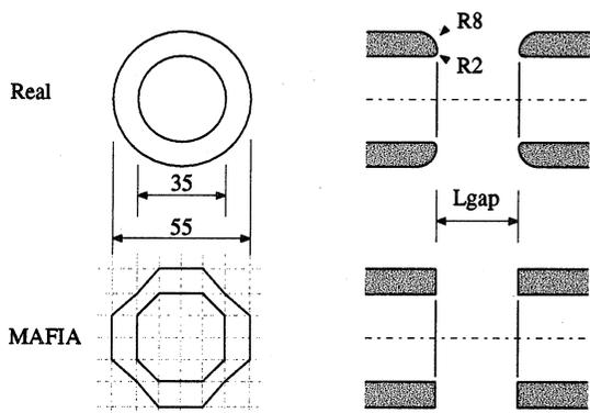
Figure 2: The real drift tube and its substitute. The octagonal cross section is discretized with three radial cells.
