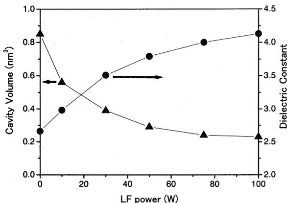
Figure 3: Cavity volume (triangles) and dielectric constant (circles) vs. LF power of the PECVD process.
