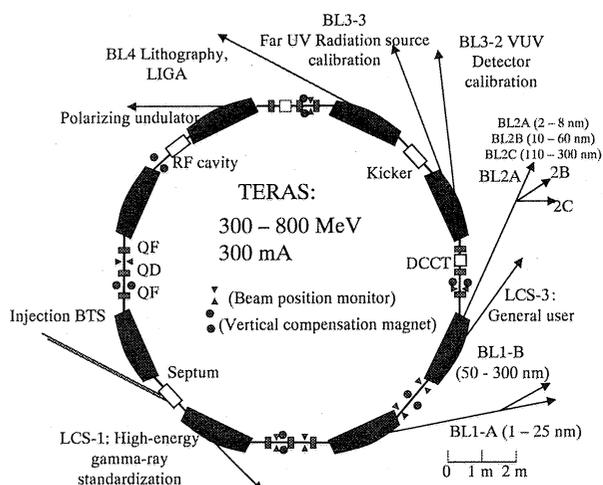
Figure 4: Plan view of storage ring TERAS.
