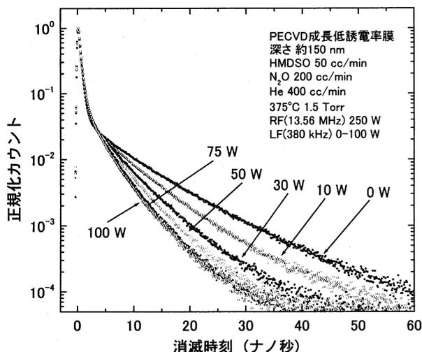
Figure 2: Positron lifetime distributions for the hexamethyldisiloxane-based thin films formed by dual-frequency PECVD.
