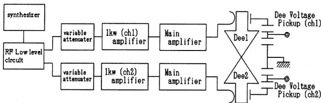
Figure.4 : RF system of NIRS-930
