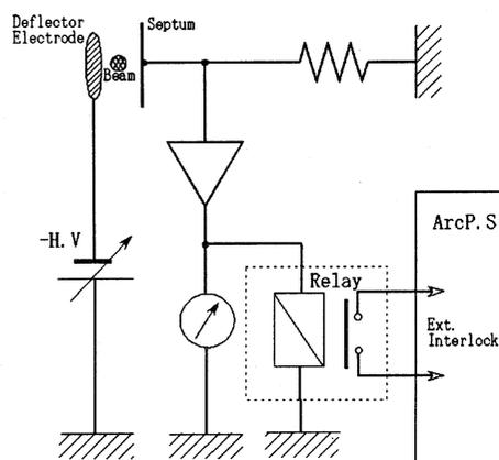
Figure.2 : Block diagram of floating septum system.
