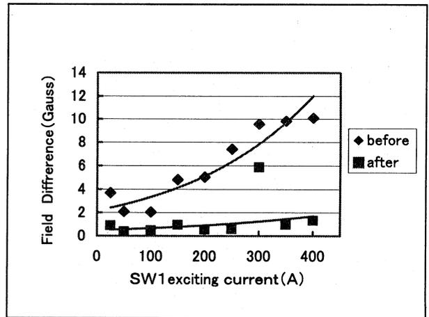
Figure.5 : The field differences inside of the SW1.
