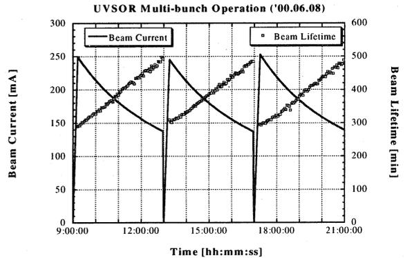
Fig.1 Typical beam current history in multi-bunch mode
