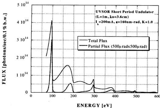
Fig. 2 The expected SR spectra from the in-vacuum undulator
