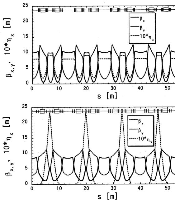
Fig. 6. Optical functions of present (lower) and upgraded (upper) lattice
