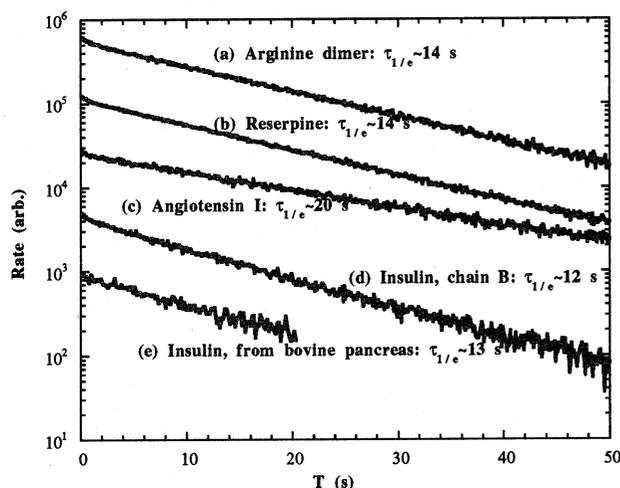
Figure 7. Time dependence of the neutral beam production rates for 20-keV/charge bio-molecular ions: (a) arginine dimer (charge, 1+; M.W., ~331), (b) reserpine (1+; ~609), (c) angiotensin (1+; ~1298), (d) insulin chain B (3+, ~3499) and (e) insulin from bovine pancreas (5+; ~5738). The 1/e lifetimes are indicated in the figure. The vacuum pressure was about  $4 \times 10^{-11}$  Torr. The decay curves are arbitrarily scaled in magnitude to facilitate a comparison.
