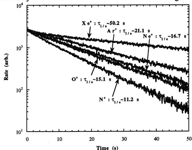
Figure 6. Time dependence of the neutral beam production rate for 20-keV atomic ions at an injected current of 10~20 nA. The vacuum pressure was about  $3 \times 10^{-11}$  Torr. The decay curves are arbitrarily scaled in magnitude to facilitate a comparison [4].
