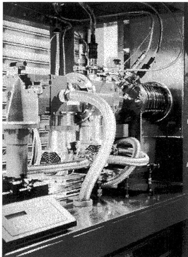
Figure 3 . Photograph of the electro spray ion source.
