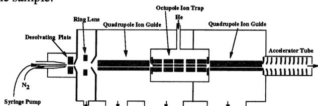
Figure 2. Schematic drawing of the electro spray ion source, ion guides and an ion trap.
