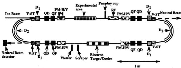
Figure 4. Layout of the electrostatic storage ring. D<sub>1</sub> and D<sub>2</sub> indicate 10° and 160° deflectors, QF and QD the horizontally focusing and defocusing electrostatic quadrupoles, PM-H and PM-V the horizontal and vertical position monitors, RF the drift-tube RF system and V-ST the vertical steerer.
