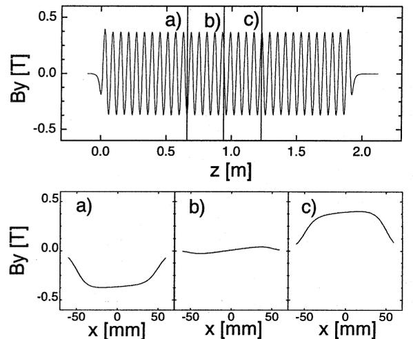
Figure 3: Magnetic field calculated with parameters listed in Table 1 and edge angle  $\phi = 2^\circ$ . a), b) and c) shows the positions where transverse variation of the magnetic field in the lower panel are calculated.
