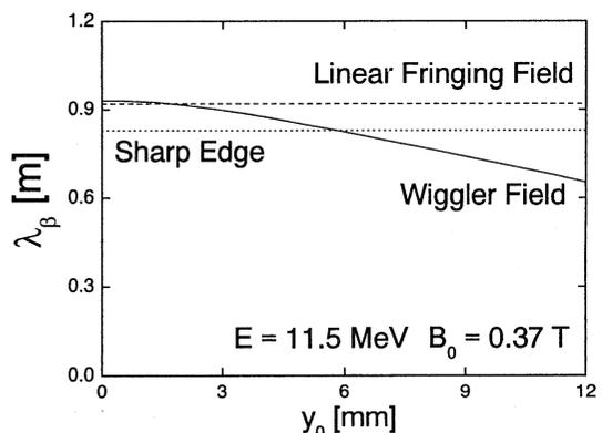
Figure 1: Betatron wavelength  $\lambda_\beta$  calculated as a function of the oscillation amplitude  $y_0$ .
