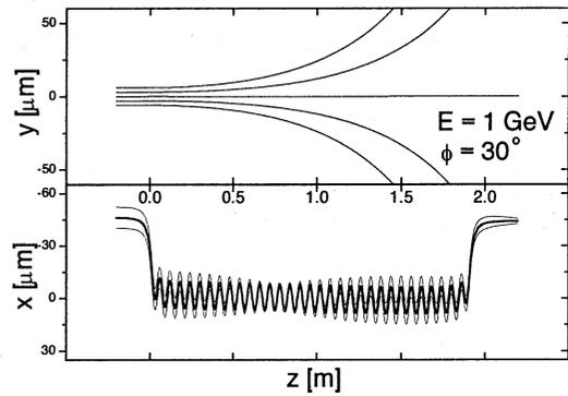
Figure 6: Trajectories of the 1 GeV electron in the EF wiggler with  $\phi = 30^\circ$ .
