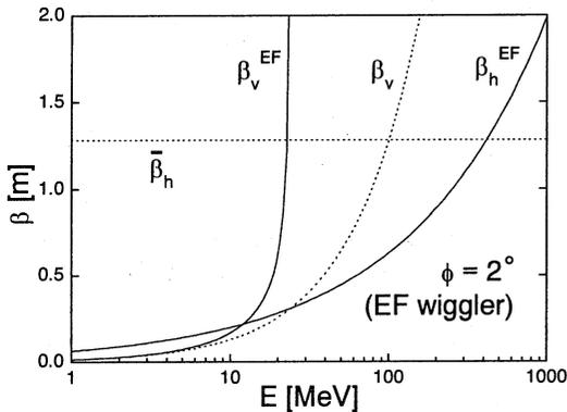
Figure 5: Betatron function as a function of electron energy. See text in details.
