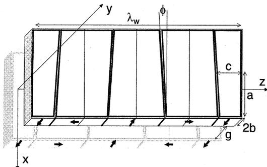
Figure 2. Schematic drawing of a single period of the Edge Focusing (EF) Wiggler.
