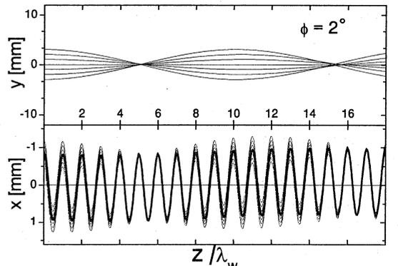
Figure 4: Trajectories of the 11.5 MeV electron calculated with the field shown in Fig. 3.
