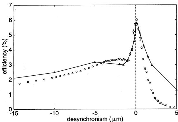
Figure 3: The open-circles are typical efficiencies as a function of detuning length in JAERI-FEL [4]. The solid-triangles are our numerical results [10], which agree with the measured efficiency curve well. The solid-line is a guide to the eye.
