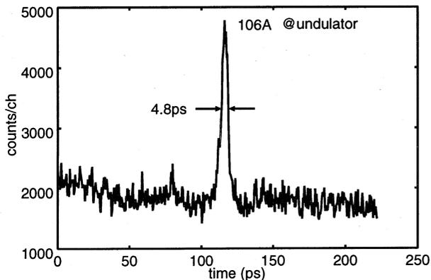
Figure 2: A synchroscan streak camera signal obtained at the center of the undulator.
