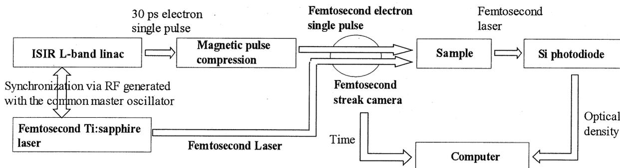
Figure 1. Diagram of subpicosecond pulse radiolysis system
