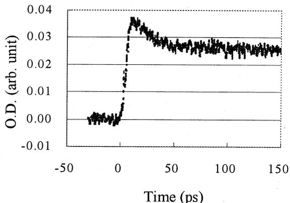
**Figure 5.** The time-dependent behavior of intermediates generated in neat methanol, measured with the newly-developed subpicosecond pulse radiolysis system at the wavelength of 790 nm.
