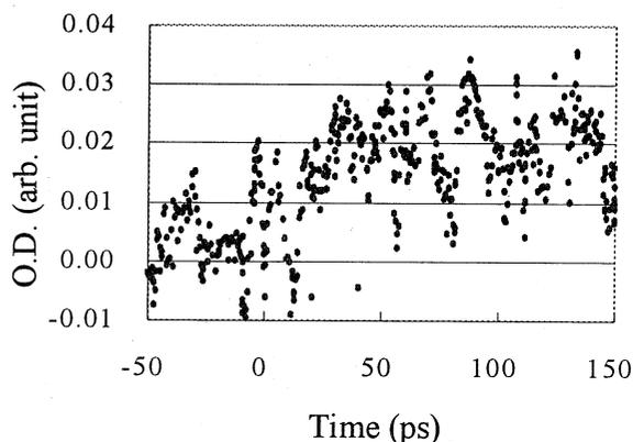
**Figure 4.** The time-dependent behavior of intermediates generated in neat methanol, measured with the previous subpicosecond pulse radiolysis system at the wavelength of 790 nm.
