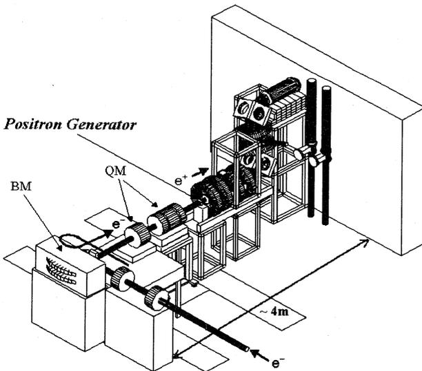
Figure 3: Design of the beam line
