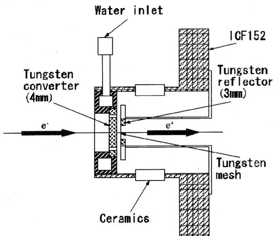
Figure 5: Design of the positron generator
