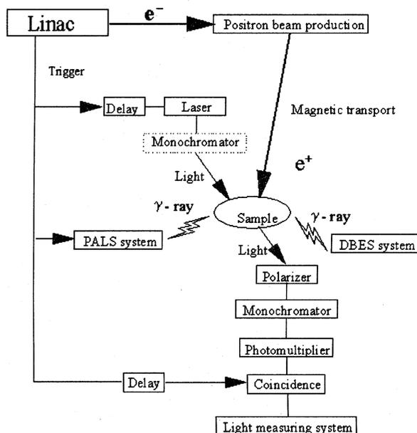
Figure 1: Measuring system based on the L-band linac.
