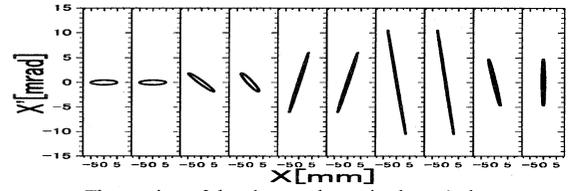
The motion of the electron beam in the  $xx'$  phase space
