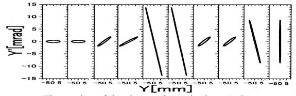
The motion of the electron beam in the  $yy'$  phase space
