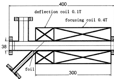
Fig.1 Layout of laser tube and solenoid coils
