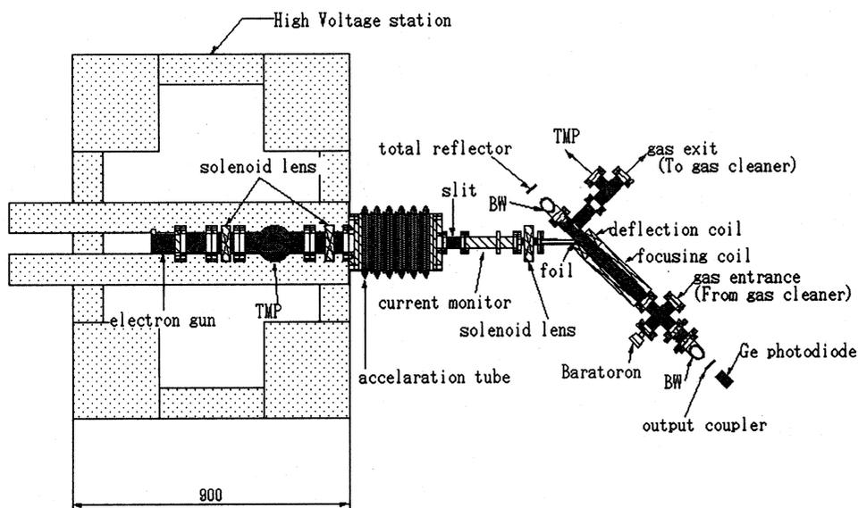
Fig5 Schematic of the experimental setup
