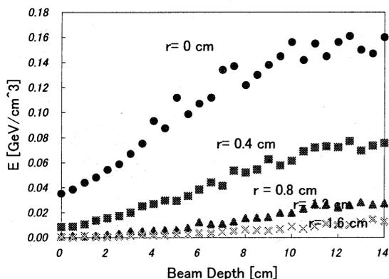
Figure 3: The distribution of the energy deposition
