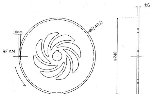
Figure 2: A drawing of one target sheet
