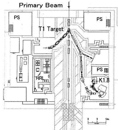
Figure 1: The floor plan of the K-Hall and T1 target
