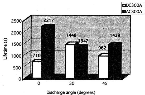
Fig. 4: C-foil lifetime dependence on the angle between the direction of arc discharge and the horizontal plane.
