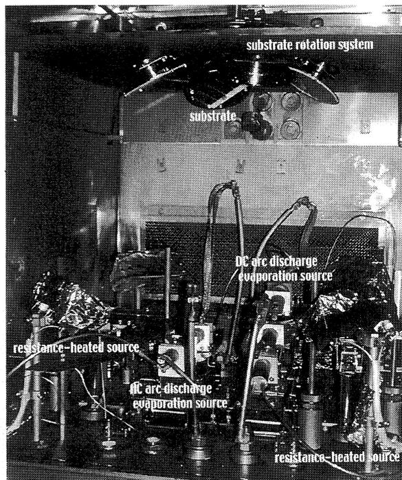
Fig. 2: The inside view of vacuum chamber.
