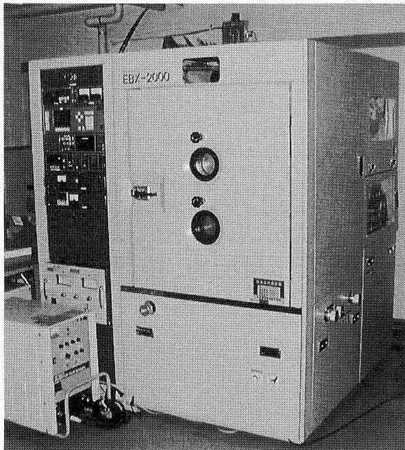
Fig. 1: High vacuum evaporation system (EBX-2000C by ULVAC).
