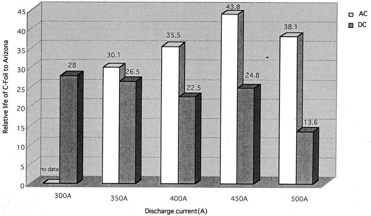
Fig. 5: The dependence of C-foil lifetime on the discharge current.
