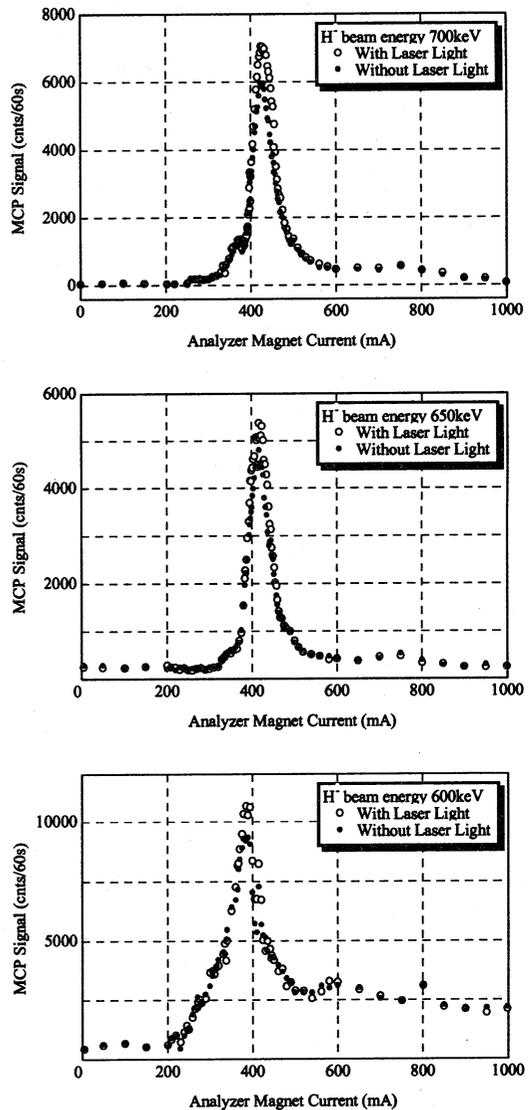
Figure 3: Characteristics of the MCP signal by changing the coil current of the analyzer magnet. The position of this peaks depended on the energy of the H beam. During these measurement, the retarding voltage was set to -100 V to reject the low-velocity electron component.
