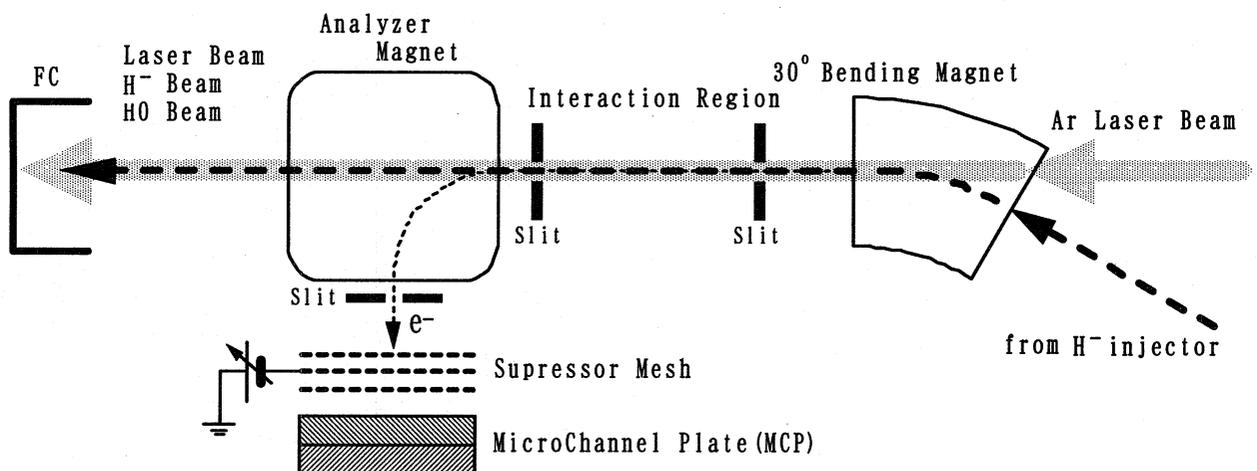
Figure 1: Schematic diagram of the energy analysing system for electrons photodetached from a  $H^-$  beam using an Ar laser beam.
