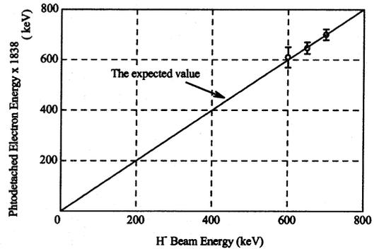
Figure 7: Correlation between the H beam energy and the photodetached electron energy by retarding method. The plotted points are the data obtained from Fig. 6.
