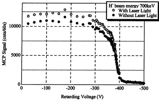
Figure 4: Characteristics of the MCP signal by changing the retarding voltage, when the H beam energy was kept to 700 keV.
