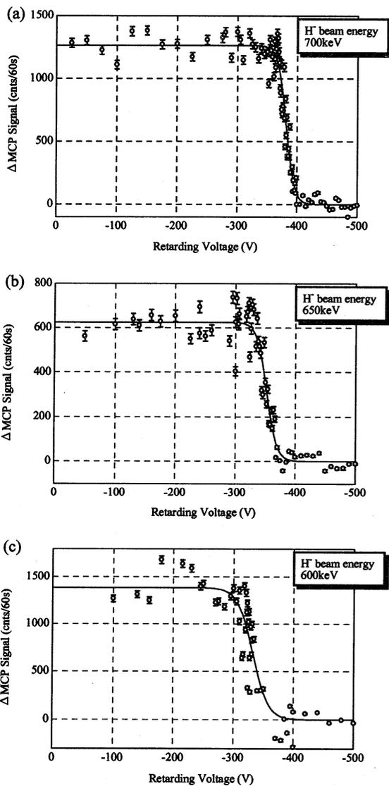
Figure 5: The difference between data with/without laser beam versus retarding voltage. H beam energies were set to (a) 700 keV, (b) 650 keV and (c) 600 keV, respectively.
