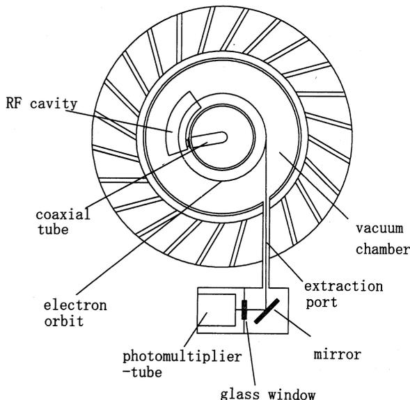
Figure 1 : Cross section of the AURORA ring showing the electron orbit and the RF cavity. The RF power is transmitted from below through the coaxial tube. Photomultiplier-tube is used to measure the power of the radiation beam.
