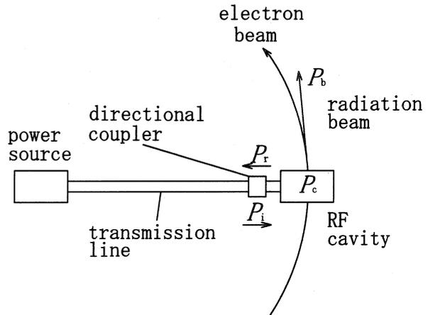
Figure 2: Power flow in the accelerating system of the AURORA ring.  $P_i$  is the supplied power,  $P_b$  the beam loading,  $P_c$  the wall loss of the RF cavity,  $P_r$  the reflection loss of the RF cavity, and  $P_e$  the transmission loss.
