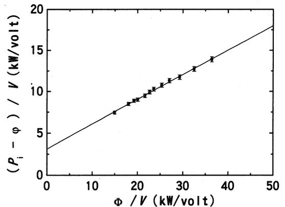
Figure 3: Plot of  $(P_i - \phi) / V$  against  $\Phi / V$  with changing the magnitude of stored beam current. A linear relation holds, showing that the assumption on the conservation of the RF power is correct. Magnitudes of error are indicated by the error bar. The error in  $\Phi / V$  is smaller than the diameter of the solid circle.
