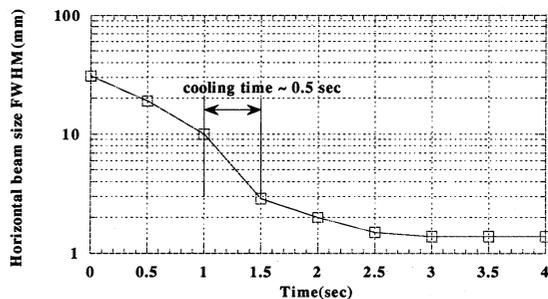
Fig. 3: Compressing horizontal beam-size (FWHM) as a function of time.
