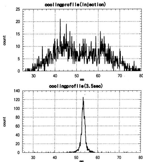
Fig. 2: Upper figure: Horizontal beam-profile with FWHM of around 30 mm just after multiturn injection. Lower: that with FWHM of 4 mm after cooling of 3.5 sec.
