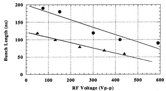
Fig. 7: The rf-voltage dependency of the bunch width. Circles and triangles indicate bunch width in the sinusoidal rf-field and in sawtooth-wave one, respectively.
