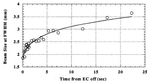
Fig. 4: The beam-size growth due to IBS after switching the electron beam off. Circles are measured ion-beam size. Solid line indicates the fitting result by the analytical formula.
