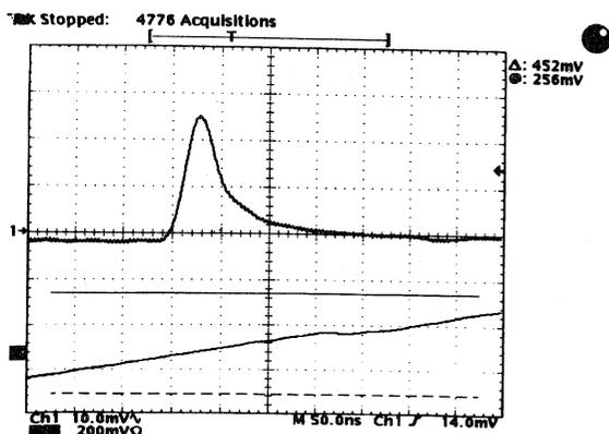
Fig. 6: Bunch shape in cooling and applying sawtooth-wave rf-field. Horizontal scale is 50 ns/div.
