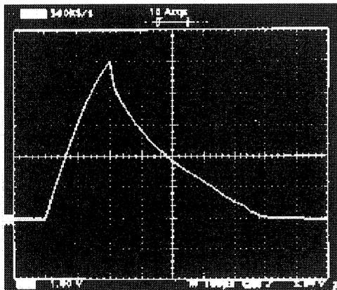
Figure 3: typical controlled-decay waveform.
