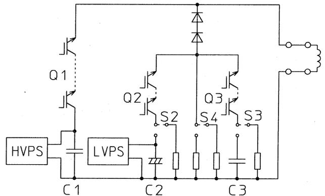
Figure 1: Schematic of main circuit.
