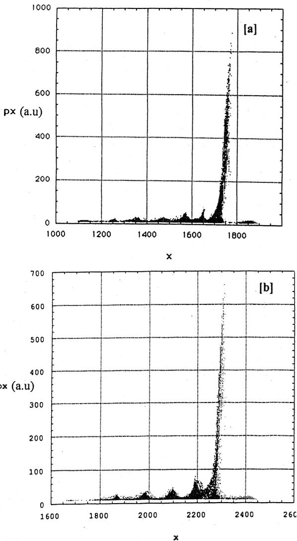
Fig. 4. Longitudinal phase space plot for trapped electrons in case of  $a = 4$ . (a) the laser pulse propagating in an inhomogeneous plasma. (b) the pulse propagating only in homogeneous plasma.
