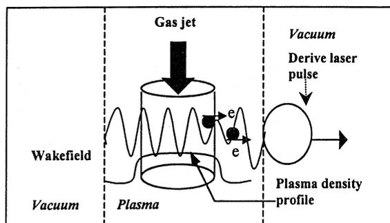
Fig.1. Schematic of the plasma cathode by using single laser beam and wavebreaking injection of plasma electrons. The plasma density profile is adjusted using a specially designed gas jet. In the region of density inhomogeneity the wakefield is locally decayed, hence the plasma electrons are pre-accelerated and injected into the regular region of the wakefield for more acceleration. Our experiment will be based on this scheme.
