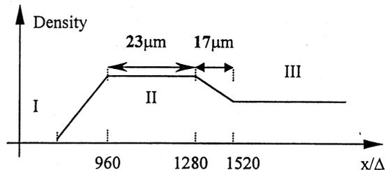
Fig.2. Schematic of the plasma density profile for our simulations, the simulation delta  $\Delta = 0.072 \mu\text{m}$ .
