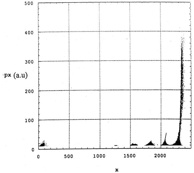
Fig.5. Phase space for trapped electrons in inhomogeneous plasma for the case of  $a = 2.6$ , 12 TW, 50 fs laser pulse.
