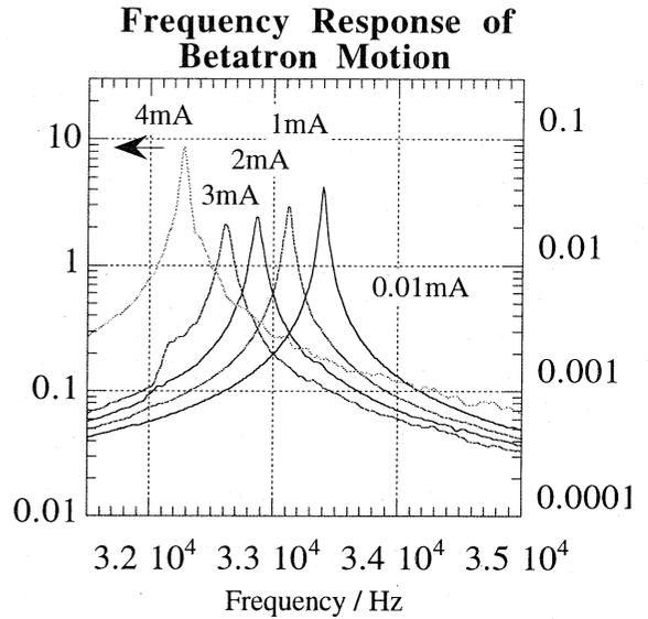
Fig. 6 Frequency response of the vertical betatron motion at chromaticity 0.23.
