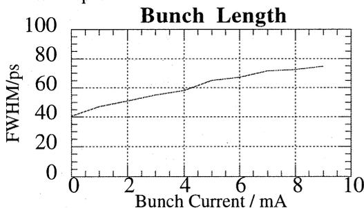
Fig. 1 Bunch length vs. Bunch current
