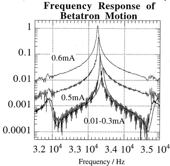
Fig. 4 Frequency response of the vertical betatron motion at chromaticity -4.
