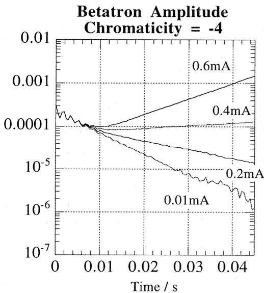
Fig. 5 Betatron amplitude growth vs. bunch current. The bunch current is increased as in Fig. 3. The growth rate of the instability is gradually increased as the bunch current.
