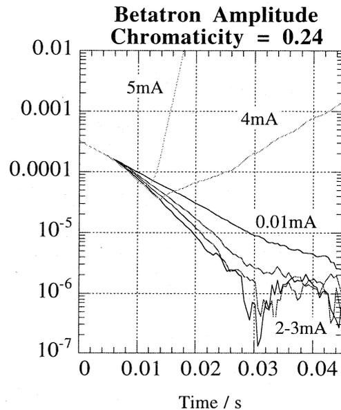
Fig. 7 Betatron amplitude growth vs. bunch current. The bunch current is increased as in Fig. 3. The growth rate of the instability is suddenly increased at threshold bunch current. At low bunch current, the head-tail damping can be seen.
