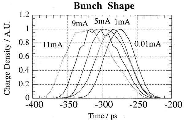
Fig. 2 Bunch shape vs. bunch current.
