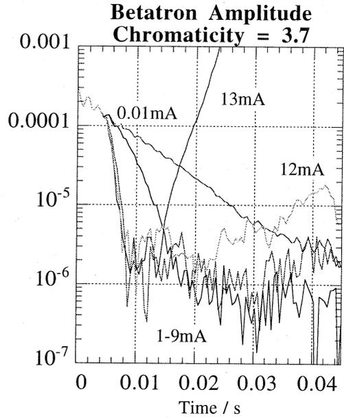
Fig. 10 Betatron amplitude growth vs. bunch current. The bunch current is increased as in Fig. 3.
