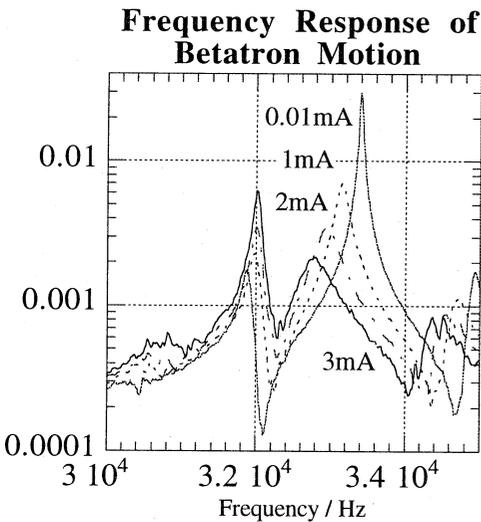
Fig. 9 Frequency response of the vertical betatron motion at chromaticity 3.7.
