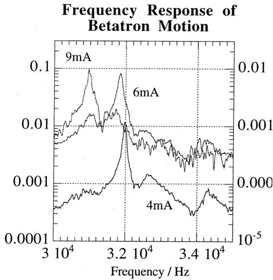
Fig. 8 Frequency response of the vertical betatron motion at chromaticity 3.7
