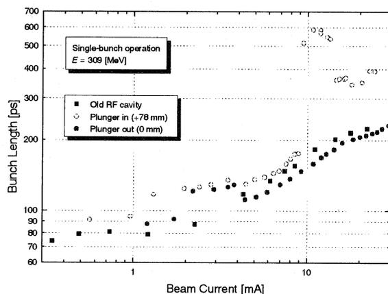
Fig. 5 Dependence of the bunch length on the beam current.
