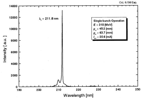
Fig. 3 A spectrum of the shortest-wavelength FEL
