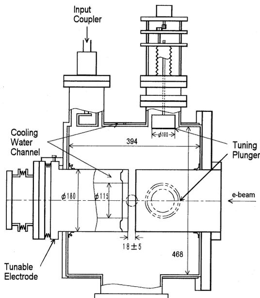
Fig. 4 Overview of the new RF cavity
