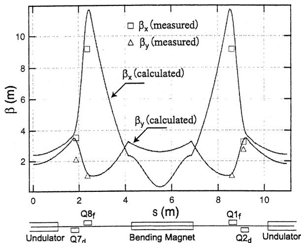
Fig.5 The betatron function of HiSOR storage ring, measured and calculated.
