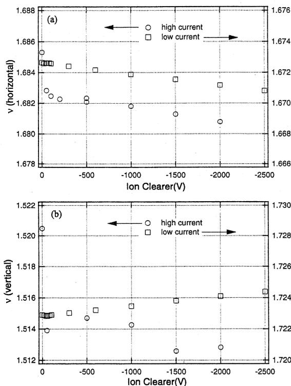
Fig.4 Tunes when ion clearer voltage is changed.
