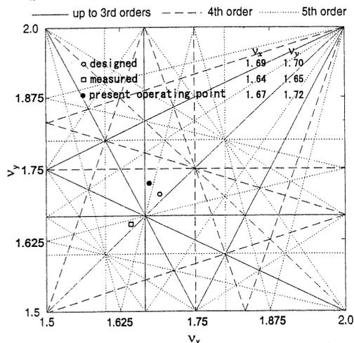
Fig.2 Tune diagram of HiSOR storage ring.
