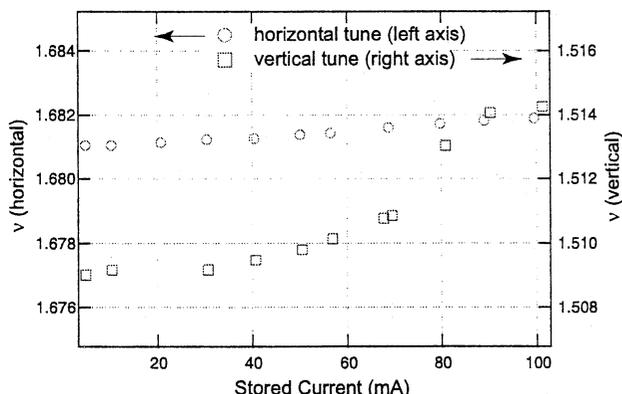
Fig.3 Beam-current dependence of the tune
