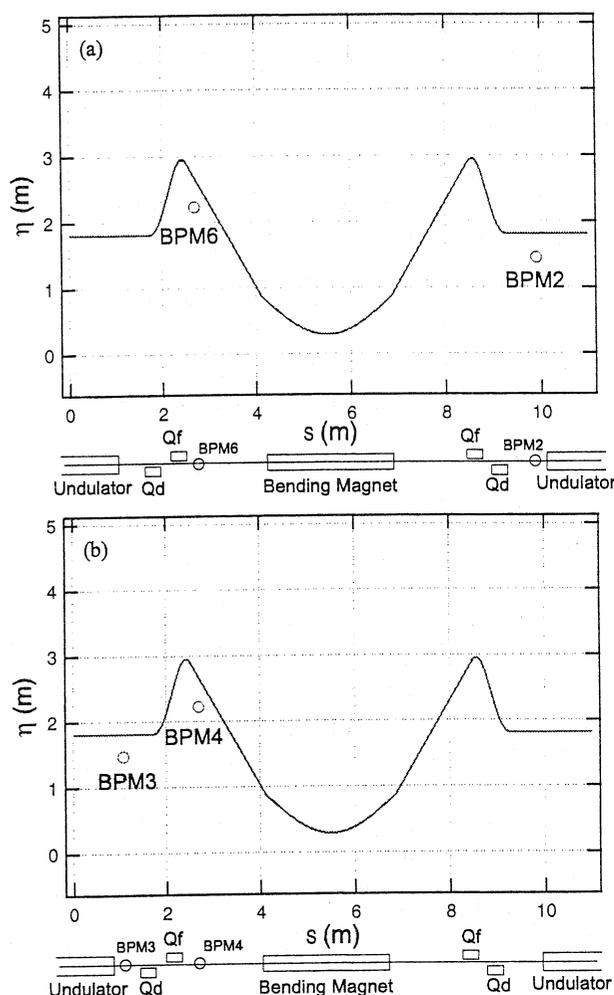
Fig.6 The eta function of HiSOR storage ring, measured and calculated.
