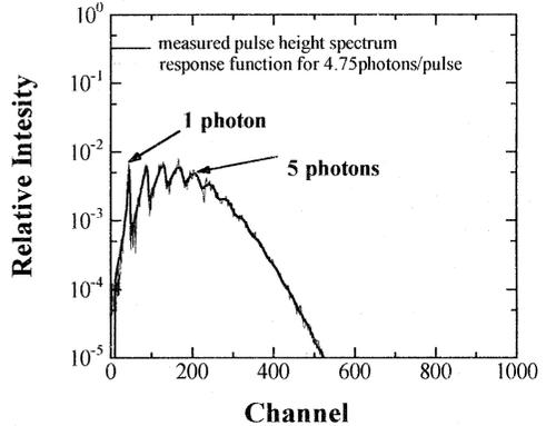
Fig. 5 Measured pulse height spectrum (thick line) and response function (thin line).
