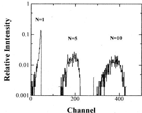
Fig.1 The gamma ray response function of the BGO scintillation detector for the multi-photon injection.  $N$  is the number of the photon injected to the detector.
