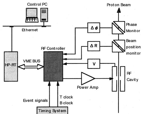
Fig.1 A block diagram of the RF control system.
