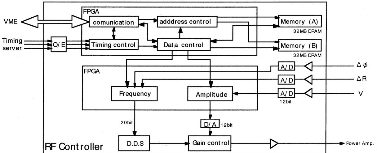
Fig.2 A block diagram of the RF Controller
