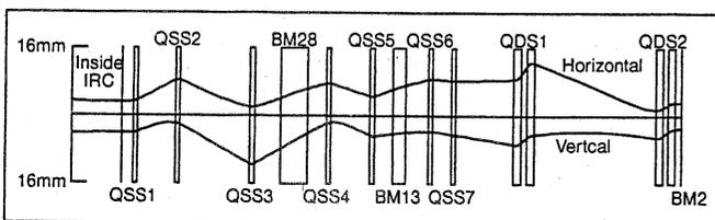
Fig.3 Beam envelope calculated for the beam line from the IRC to the SRC.
