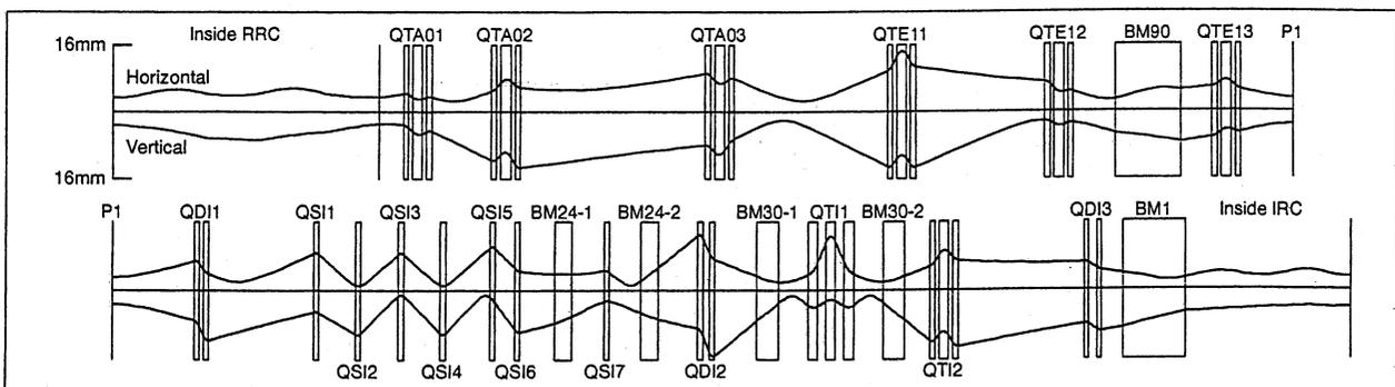
Fig.2 Beam envelope calculated for the beam line from RRC to IRC. A first-order ion-optical calculation was performed. The beam emittance is  $5\pi \text{ mm}\cdot\text{mrad}$  and the momentum spread is  $\pm 0.05\%$  in this calculation.
