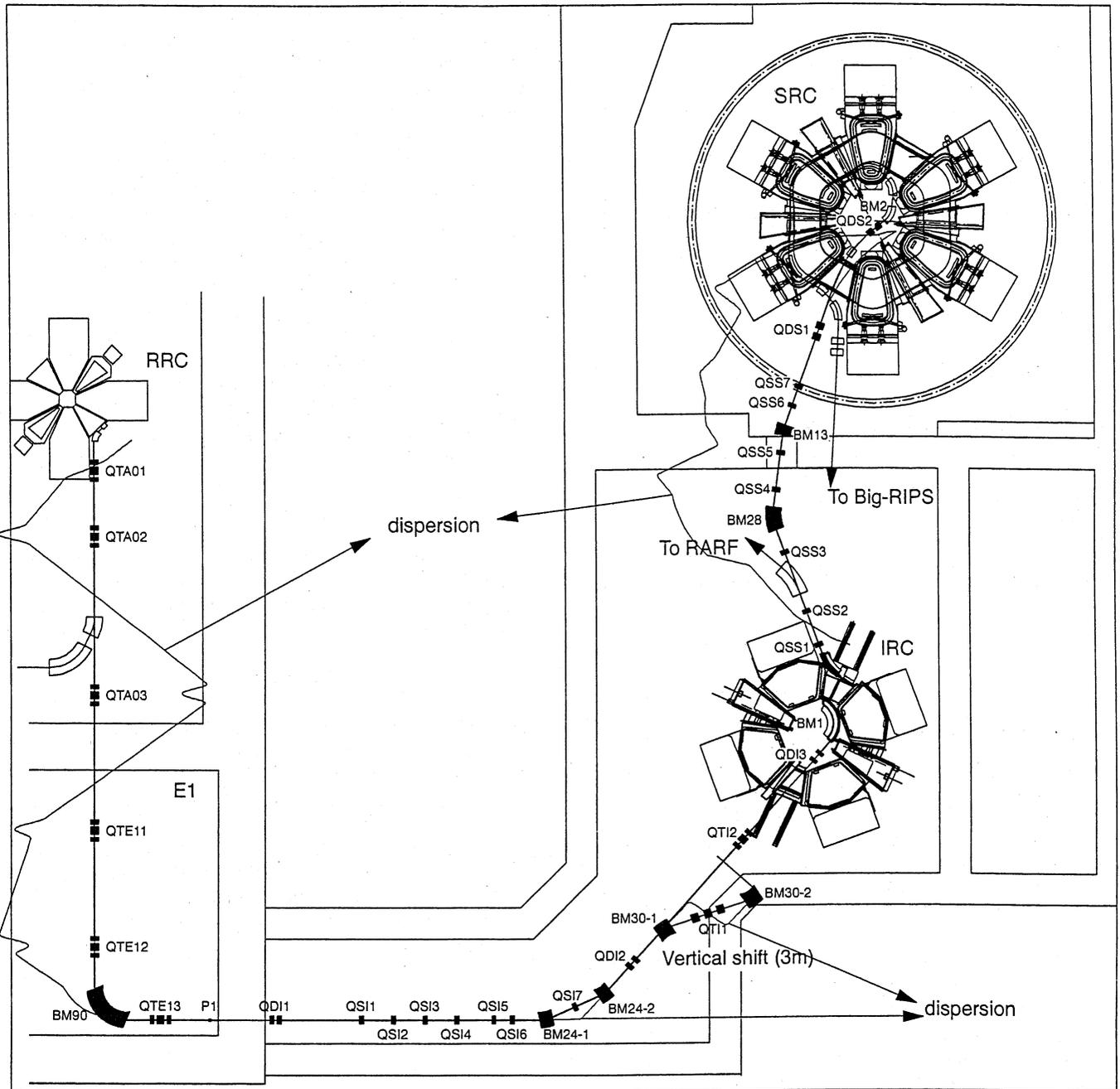
Fig.1 Rayout of the beam transport system in the RI Beam Factory. The scale is 1/400.
