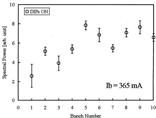
Fig.4 Spectral powers of leading 10 bunches with the DIPs ON.
