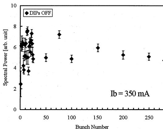
Fig.3-a Spectral powers of bunches with the DIPs OFF.
