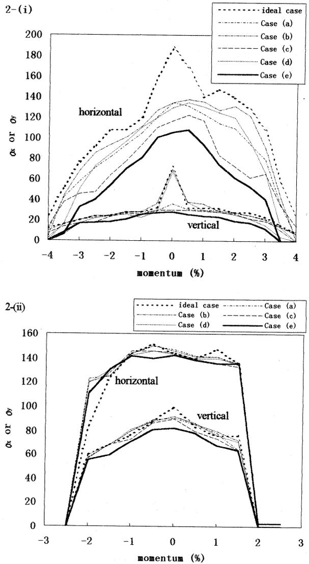
Fig. 2 Dynamic apertures after correction in various cases. Figure 2-(i) is for low emittance mode, and Figure 2-(ii) for high emittance mode. The  $\sigma_x$  and  $\sigma_y$  are defined as,
