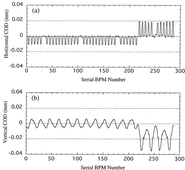
Fig. 6 Simulated horizontal (a) and vertical (b) COD. (a) The momentum change caused by 0.01 % reduction of field strength of dipole magnets in D-zone was found. (b) 0.77 μrad kicks are assumed to be distributed to every QF magnet in D-zone.
