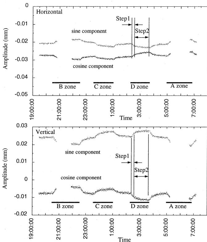
Fig. 3 Amplitude of Fourier components of COD whose harmonic number is 1 in horizontal (above) and vertical (below) directions.
