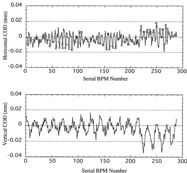
Fig. 5 Change of COD in horizontal (above) and vertical (below) directions at 95 minutes past after the temperature of cooling water at D-zone was raised to +32°C. Large open circles show the orbit at BPMs located in dispersive sections.
