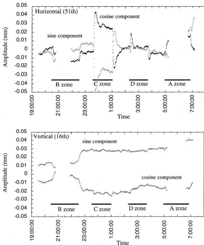
Fig. 2 Amplitude of Fourier components of COD whose harmonic number is betatron tunes in horizontal (above) and vertical (below) directions. Thick solid lines indicate periods when the temperature of the cooling water at each zone was raised to  $32^\circ\text{C}$ .
