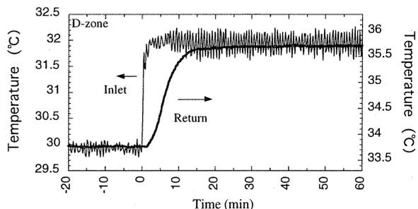
Fig. 1 A typical time dependence of the temperature rise of cooling water. The water temperature was measured at the inlet to each zone and the return from that in the circuit.
