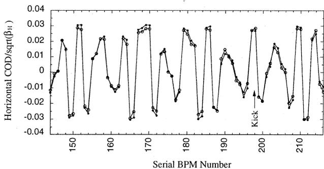
Fig. 4 Measured (open circle) and simulated (solid circle) orbit distortion in horizontal direction in a quarter of the ring. Simulated orbit was calculated with +5.6  $\mu\text{rad}$  single kick between BPM No. 197 and 198.
