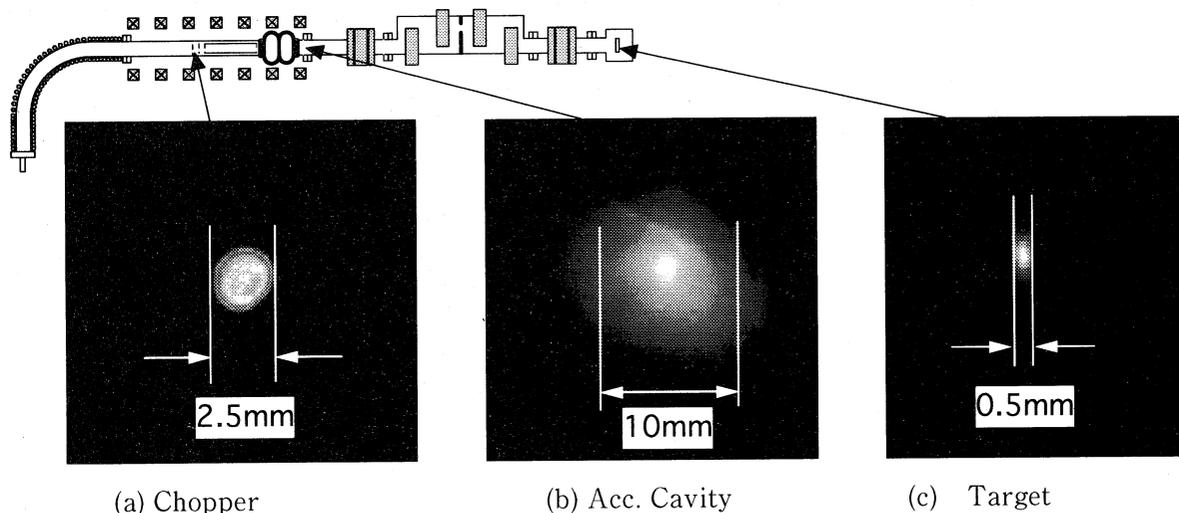
Fig.3 Beam Profiles
