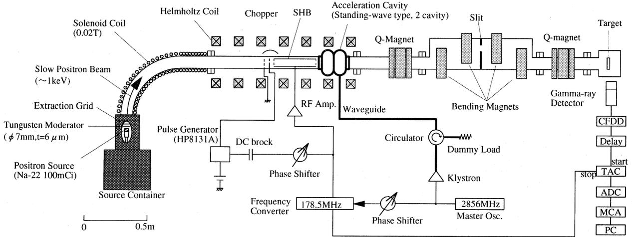
Fig.1 Schematic of PUMPS
