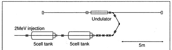
Fig. 1 The layout of JAERI-FEL accelerator room (July 1999).
