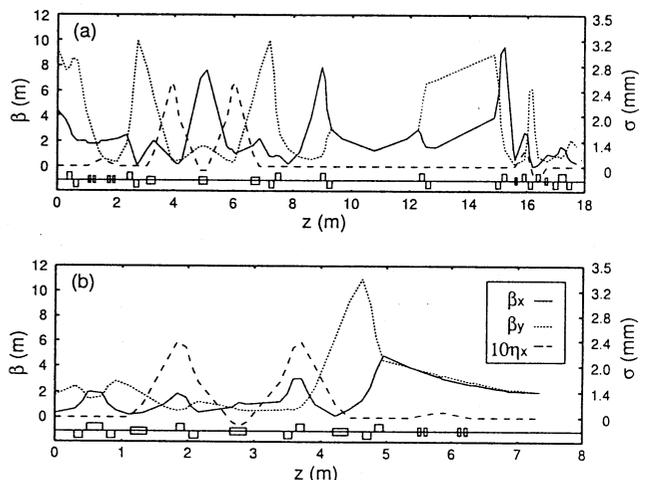
Fig. 3 Betatron function and dispersion function during the designed recirculation: (a) from the accelerator to the undulator and (b) from the undulator to the accelerator.
