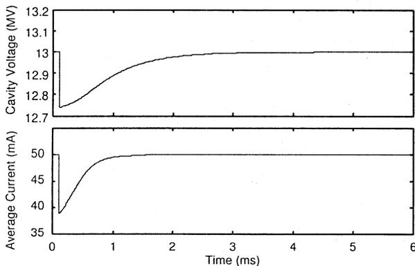
Fig. 4 Time profile of cavity voltage and average beam current. (2% perturbation is applied to the cavity voltage at  $t = 0.1$ ms.)
