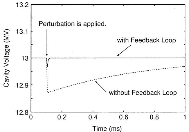
Fig. 5 RF field stabilization with a feedback loop.
