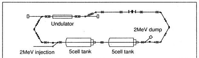
Fig. 2 The layout of JAERI-FEL accelerator room for the energy-recovery experiment.
