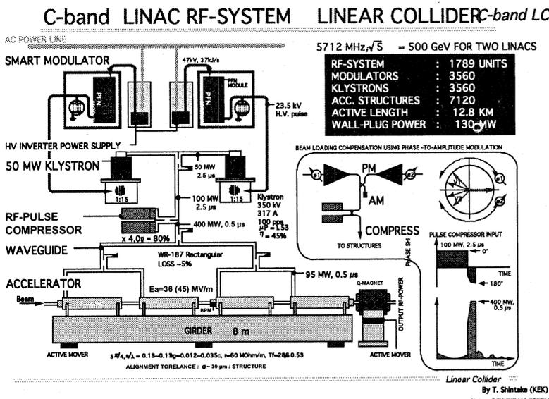
Fig. 1: One unit of the C-band main linac.
