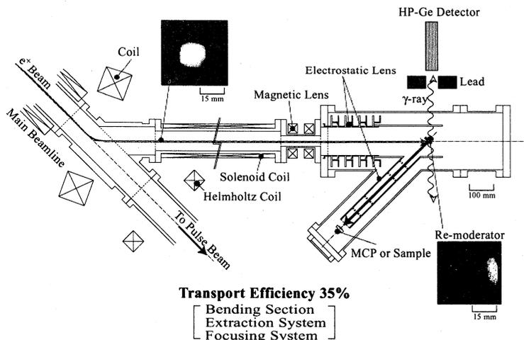
Figure 3. Experimental setup and data of the brightness enhancement experiment.
