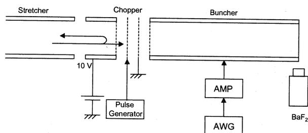
Figure 4. Schematics of the bunching system.
