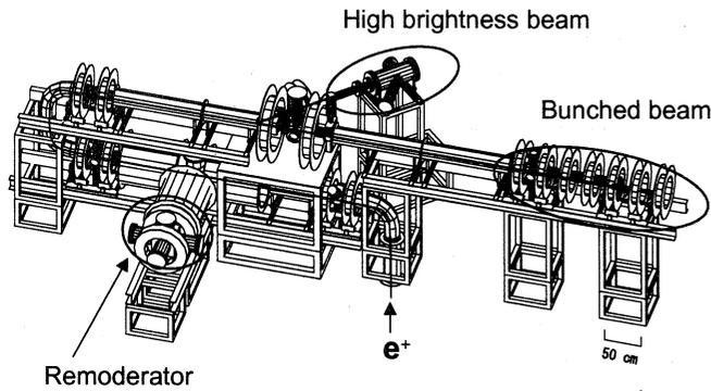
Figure 2. Schematics of the beamline in the experimental room.
