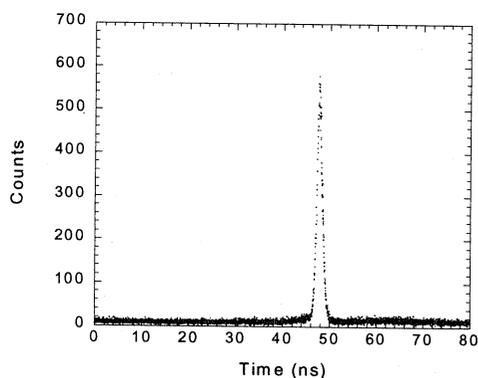
Figure 5. Time spectrum of the bunched positrons measured by annihilation  $\gamma$ -rays coming from aluminum plate.
