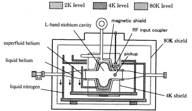
Figure 3 Cryostat for the L-band single-cell cavity
