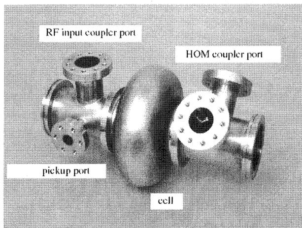
Figure 1 L-band single-cell niobium cavity
