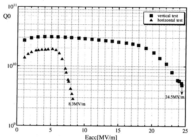
Figure 4  $Q_0$ - $E_{acc}$  plots on the single-cell cavity
