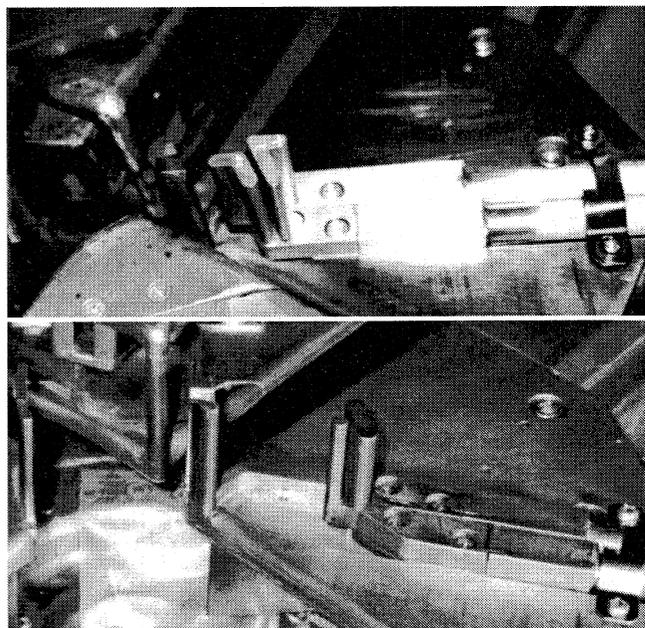
Fig. 4 Upper: a new pair of phase slit at the central region after improvement. Lower: an old phase slit before improvement.
