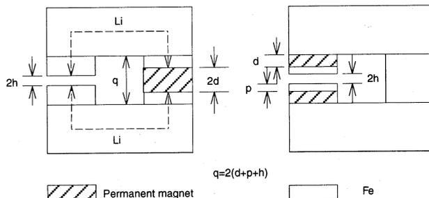
Fig.1 Geometry of the hybrid bending magnet.
