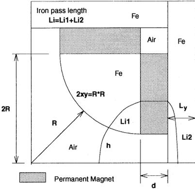
Fig.3 Geometry of 1/4 hybrid quadrupole magnet.
