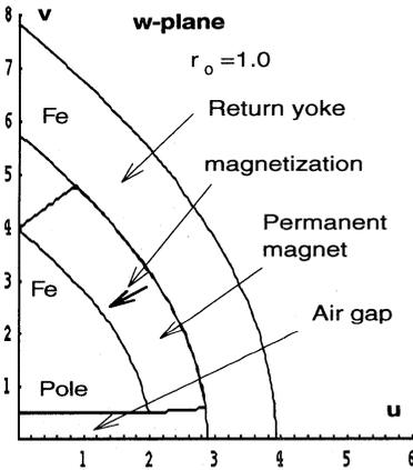
Fig.4 Transformed 1/8 quadrupole in the w-plane for the bore radius of  $R=1$ ,  $d=0.4$  and  $L_y=0.4$ .
