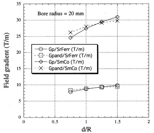
Fig.5 Comparison between the relation (11) and Pandira result.  $H_c=3.35\text{kOe}$ ,  $B_r=0.35\text{T}$  for Sr ferrite and  $H_c=10.5\text{kOe}$ ,  $B_r=11.0\text{T}$  for SmCo. Subscripts "pand" and "p" mean results by Pandira code and analytic formula, respectively.
