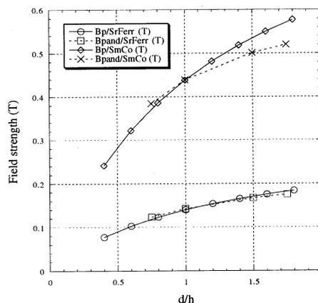
Fig.2 Field strength obtained by the simple formula and Pandira code.  $H_c = 3.35\text{kOe}$ ,  $B_r = 0.35\text{T}$  for Sr ferrite and  $H_c = 10.5\text{kOe}$ ,  $B_r = 11.0\text{T}$  for SmCo. Subscripts "pand" and "p" mean results by Pandira code and analytic formula, respectively.
