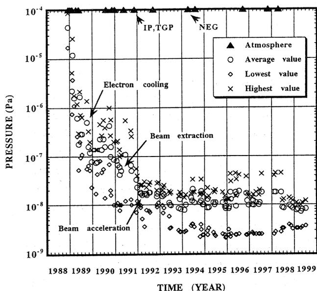
Fig. 1. Change of the vacuum pressure.
