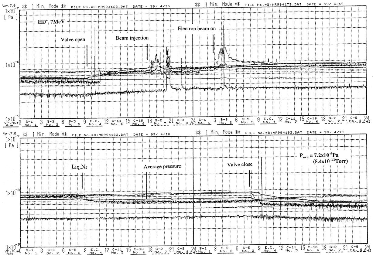
Fig.3. An example of vacuum pressure as a function of time which were measured at eight positions of a ring during the beam time. Liq.N<sub>2</sub> means that liq N<sub>2</sub> was filled up into the titanium getter chamber with liquid nitrogen trap in upstream transport line of inflector chamber.
