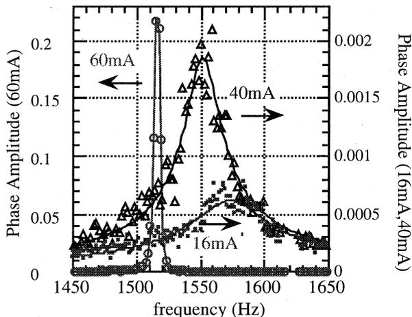
Fig. 8 Observed frequency response of the amplitude of phase oscillation of the beam with Filter B-3. The data for 60mA is 2 magnitude larger than the data at 16mA and 40mA. The damping time/rate of the synchrotron motion from the width of the data are  $5.5ms/182s^{-1}$  for 16mA,  $12ms/83s^{-1}$  for 40mA and the beam was unstable at 60mA. These values are the expected from the theory as shown in Fig. 6. The peak height is also proportional to the damping time.
