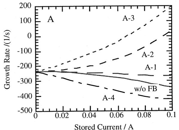
Fig. 5 Growth rate vs stored current for filter A. The growth rate includes radiation damping. The growth rate is positive above 0.6 A with the parameter B-3.
