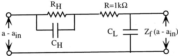
Fig. 2 The filter circuit  $Z_f$  in a feed-back controller of the SPring-8 storage ring. The values of  $R_H$ ,  $C_H$  and  $C_L$  are listed in Table 2.
