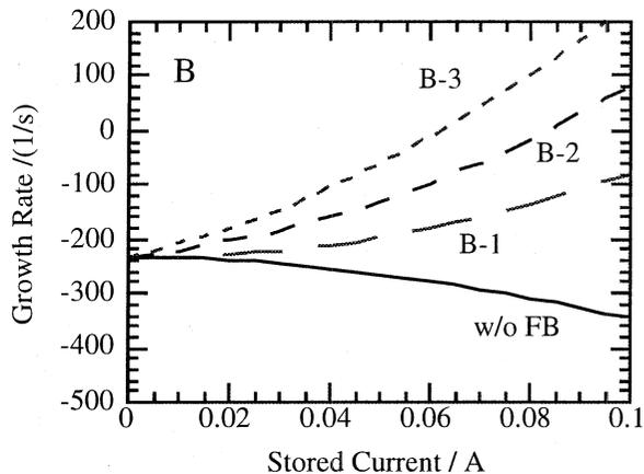
Fig. 6 Growth rate vs stored current for filter B. With B-3, Growth rate exceeds 0 at stored current more than  $\sim 0.6A$ .
