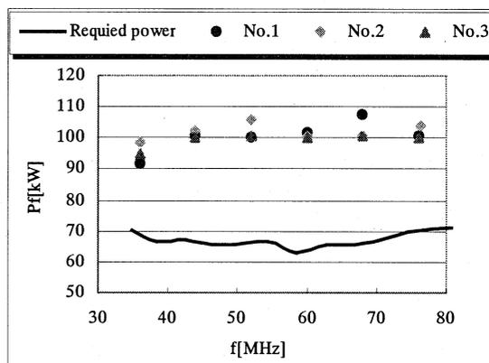
Fig.4. Maximum output power in PT and required power for CSM resonator to generate 450kV-electrode voltage. The required power was based on measurement of CSM resonator's shunt impedance..
