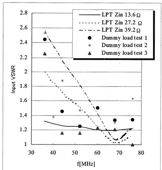
Fig.3 Input circuit's VSWR at 100kW output.
