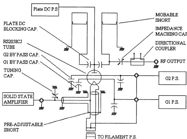
Fig.2. Schematic drawing of CSM amplifier
