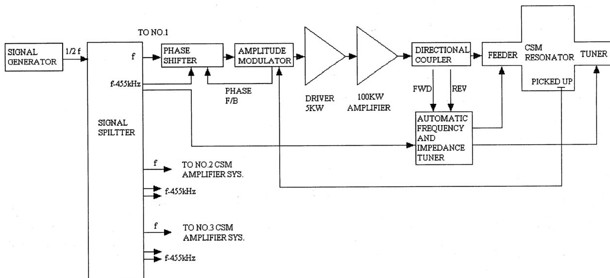
Fig.1 Block diagram of the CSM resonator and its RF feeding system
