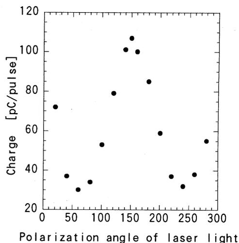
Figure.3 Bunch charge vs. Polarization angle. The angle with the maximum charge is correspondent to P-polarization.
