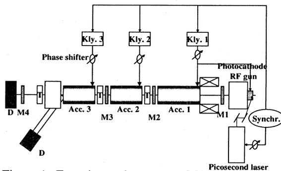
Figure.1 Experimental system. M1-4: Charge and screen monitor, T: Quadrupole Magnet, B: Bending Magnet, D: Dump
