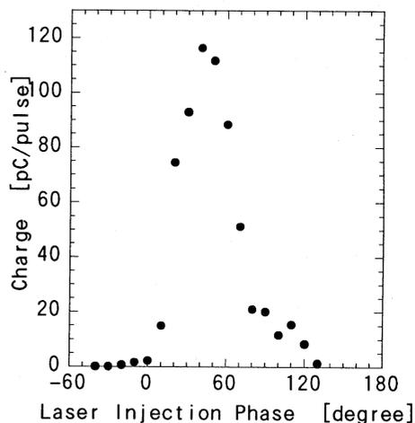
Figure.4 Emission bunch charge vs. laser injection phase. The zero point is set at charge zero phase which corresponds to the zero axial field.
