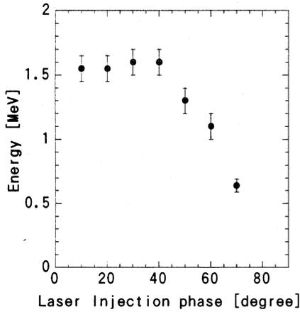
Figure.5 Electron energy from the gun
