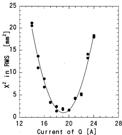
Figure 6 Square of beam diameter vs. Current of a quadrupole magnet. Solid line: Least square fitting with the 2<sup>nd</sup> order polynomial.
