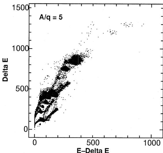
Fig. 5  $E-\Delta E$  spectrum for measurement of the cinnabar.
