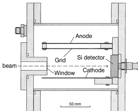
Fig. 1 Cross-sectional view of ionization chamber.
