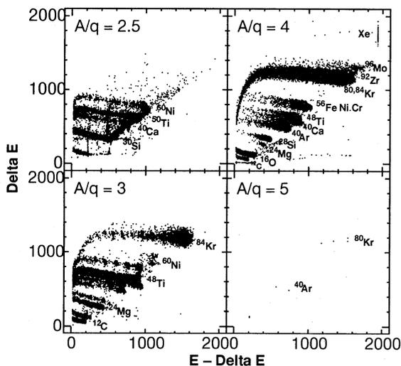
Fig. 2 E- $\Delta E$  spectra for measurement of  $\text{Al}_2\text{O}_3$  rod.
