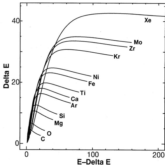
Fig. 3 E- $\Delta E$  calculation spectrum on gas pressure of 15 torr.
