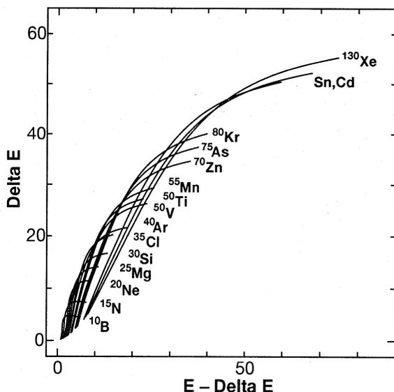
Fig. 6  $E-\Delta E$  calculation spectrum on gas pressure of 20 torr.
