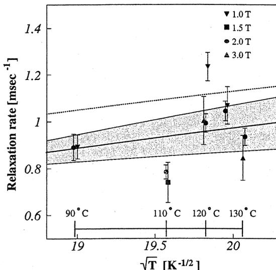
Fig. 5 Show the observed relaxation rate due to effusion effect. Hatched area shows the simulated results derived from the Monte Carlo simulation. Dotted line is derived from Eq.2.
