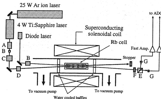
Fig. 1 Show a schematic diagram of the experimental apparatus. A pumping laser and a probe laser are injected to the Rb cell as the same direction from left to right. "A" is a Pockels cell, "B" are polarizers, "C" is a beam expander, "D" is a  $\lambda/4$  plate, "E" is a polarizing beam splitter cube, "F" is a wavelength filter, and "G" are two photo diodes.
