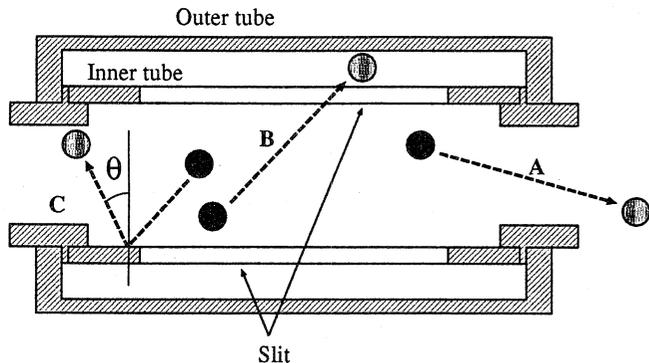
Fig. 4 Show the concept of the effusion of the polarized Rb atoms out of the pumping region. "A" is effused a Rb atom out of both sides of the cell, "B" is the effusion a Rb atom through the slits, and "C" is the bouncing of a Rb atom on the wall surface.
