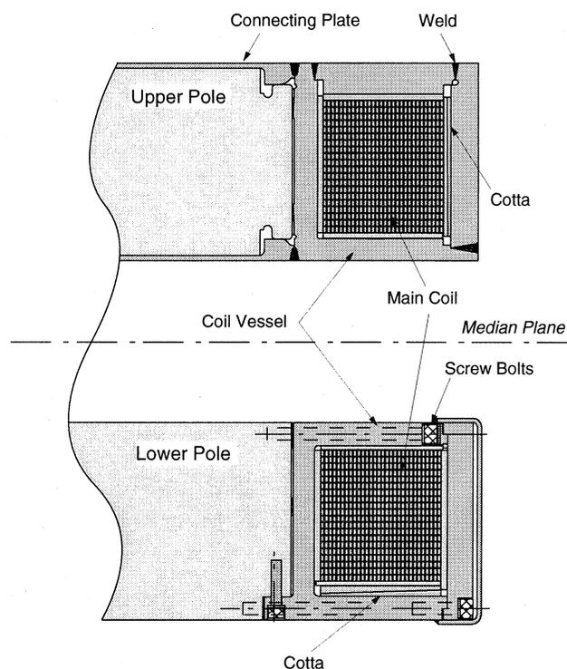
Fig. 2 Cross-sectional view of the sector magnet of the SRC.
