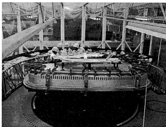
Fig. 3 Photograph of the main coil winding.
